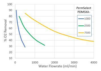
The adjacent table provides the recommended flow ranges for each degasser to provide a minimum of 50% O2 removal. So flowing at any lower flowrate will result in improved degassing. It should be noted that there is no minimum flowrate for each degasser and the flow may completely stop and go with no effects on the membrane.
